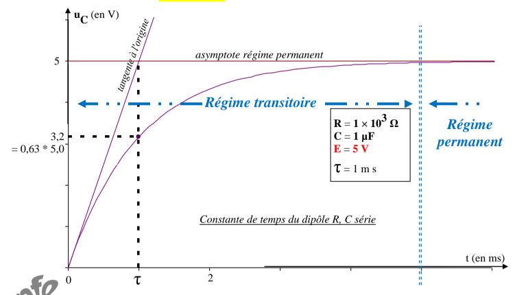
$\frac{tangente}{y = a x + b = a x} = \left(E \left(1 - e^{-\frac{t}{RC}}\right)\right)' = x = \left(\frac{E}{RC} e^{-\frac{t}{RC}}\right) = x = \frac{E}{RC} x = E \ (\hat{a} x = RC = T).$
